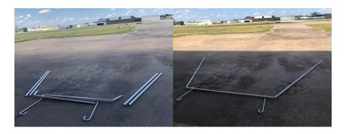
Tap the bottom pieces into the ground with the stakes in two places.....use a rubber mallet. You will see where the stakes go to hold it onto the ground. Put the other poles on top of the bottom pieces where they are swaged and crimped. Each side will have two poles. Angle the launcher so it is directly into the wind. You will put the poles away from the shore (rotate on stakes) and they lay on the ground. The whole apparatus swivels on the stakes.
